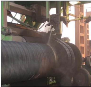
Photo.3. coating pipe gas by weight concrete in Petro jet plant, port said. Source: field study, 17 april.2019
